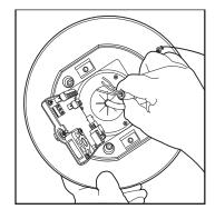
c. Pull wiring from the mount into the back box.
